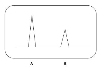
The time between the signals was 0.002 s and the distance between the microphones was 0.680 m.
