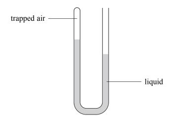
The volume V of the trapped air can be changed by changing the pressure p exerted on it.
