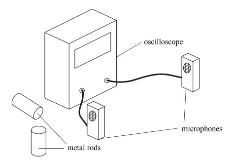
The screen of the oscilloscope showed two signals  $\bf A$  and  $\bf B$  corresponding to the sound received by the two microphones.
