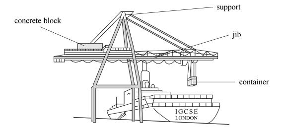
The jib is designed so that its weight is equally balanced on each side of the support. The following diagram shows the other turning forces on the jib. The jib is in equilibrium.
