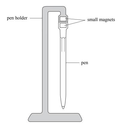
There are two ways in which the magnets can be arranged.
